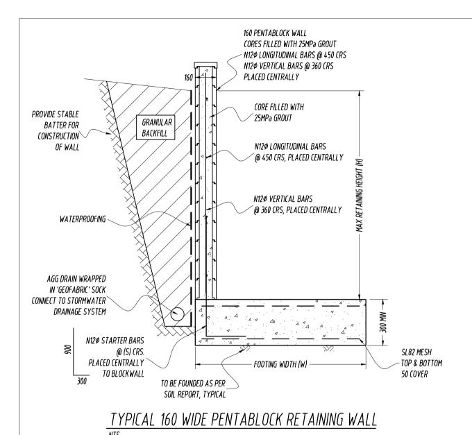
160 PENTABLOCK SYSTEM DESIGN IS BASED ON LIMIT STATE DESIGN IN ACCORDANCE WITH RELEVANT PARTS OF AS3600-2001, AS3700-2001 & AS4678-2002.
